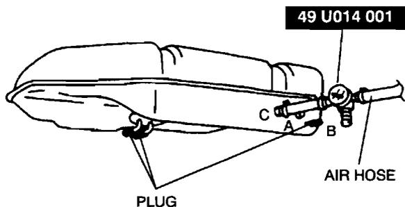
8. Apply pressure of **+0.98 kPa {+7.4 mmHg, +0.29 inHg}** to Port A and verify that there is no airflow from Port C.
