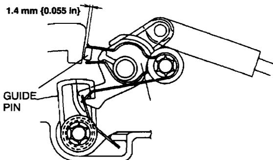
3. Clearance can be reduced by turning the cam clockwise.
