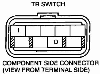
9. Adjust the switch to the point where there is continuity between the terminals.
