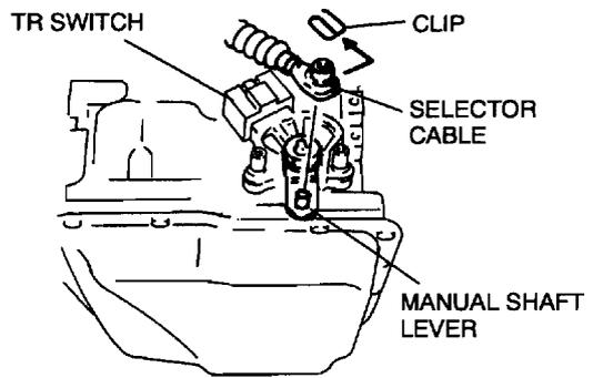
6. Remove the manual shaft nut, washer and manual shaft lever.
