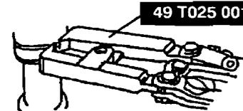
3. If clearance B is more than the specification, reduce clearance A of the SST and crimp the band again. If clearance B is less than the specification, replace the band, increase clearance A of the SST, and crimp the new dynamic damper.
