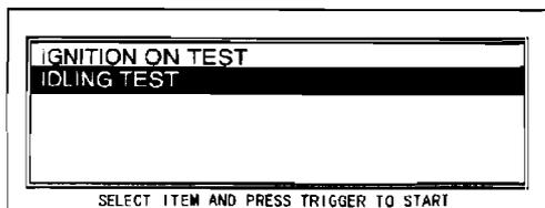
8. The screen will display PIDs. Select the appropriate PID for testing, then press the **TRIGGER** key.
