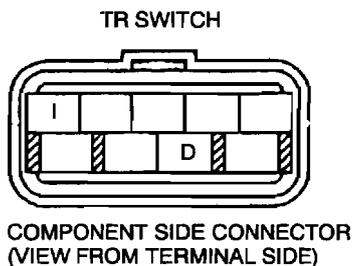
14. Adjust the switch to the point where there is continuity between the terminals.
