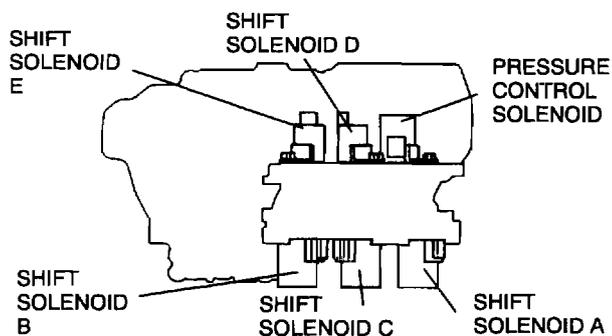
4. Apply ATF to a new O-ring and install it on the solenoid valve.
