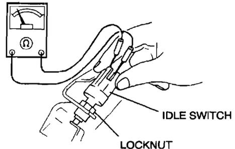
4. Press the accelerator pedal gradually by hand and verify that the output voltage of the PCM 2F terminal (accelerator position sensor) is within the specification when the output voltage of the PCM 1T terminal (idle switch) changes to B+ from below 1.0 V.
