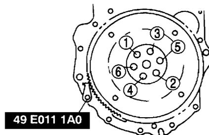
2. Remove the drive plate mounting bolts.
