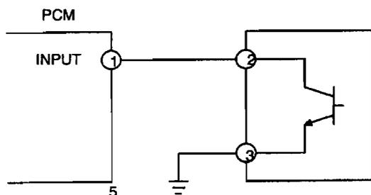
1. Measure the #1 PCM terminal voltage and confirm that it is at 0V or 5V when the ignition switch is on and the engine is at idle.
