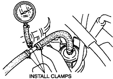
2. Measure the fuel pressure under the following conditions.
