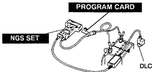
4. Select the PID/DATA MONITOR AND RECORD function on the NGS display.
