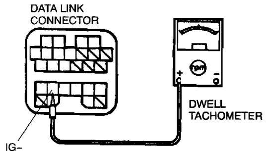
3. Verify that the idle speed is normal. (See F1-22 IDLE SPEED ADJUSTMENT.)
