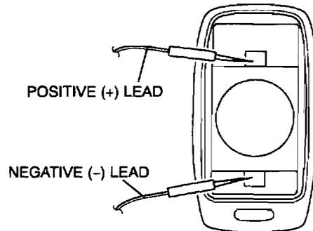
3. While pressing the battery as shown in the figure, press the LOCK and UNLOCK buttons on the transmitter at the same time for **5 seconds**.
