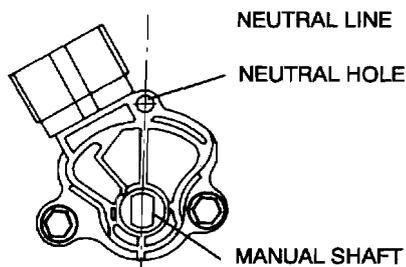
12. Hand-tighten the TR switch mounting bolts.
