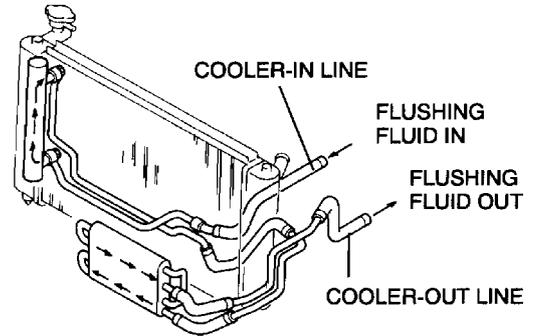
**OIL COOLER REMOVAL/INSTALLATION**
