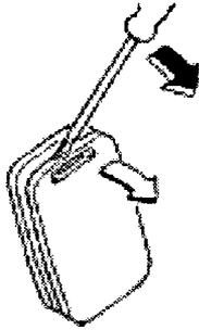
2. Press the portion of the battery indicated by A and remove the battery.
