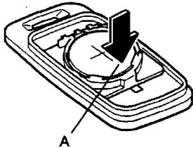
3. Install a new battery (CR2025 or the equivalent) into the front portion of the holder with the positive pole (+) facing up. Press on the B portion of the battery to set the battery.
