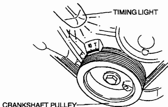
4. Increase the engine speed and verify the ignition timing is advanced.
