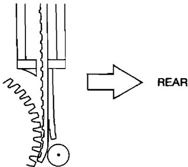
6. After the antenna mast is fully retracted, tighten the mounting nut.
