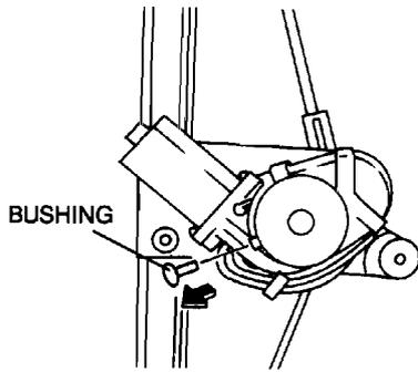
7. Slowly insert the reset jig into the hole where the bushing was installed until it stops.
