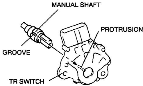
11. Turn the TR switch so that the neutral hole is in line with the flat, straight surfaces on either side of the manual shaft.
