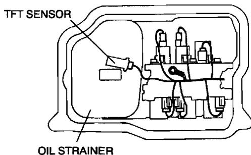
4. Install a new TFT sensor.
