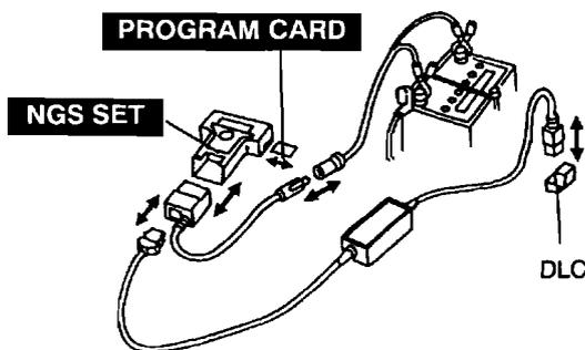
2. Connect NGS test lead (+) to the VSS connector B terminal.
