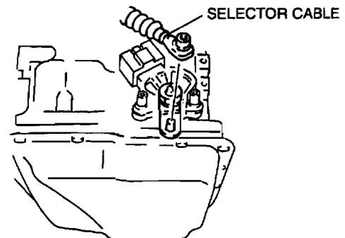
21. Inspect for continuity at the TR switch. (See TRANSAXLE RANGE (TR) SWITCH INSPECTION, Continuity Inspection.)
