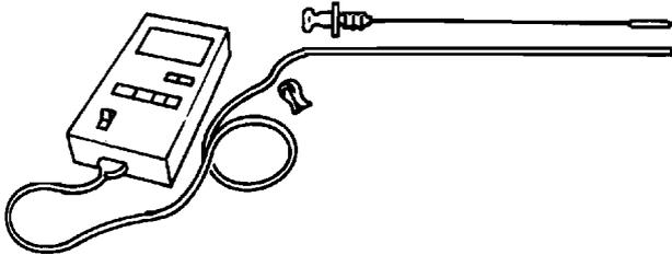
4. Warm up the engine until the ATF reaches 60—70°C {140—158°F}.
