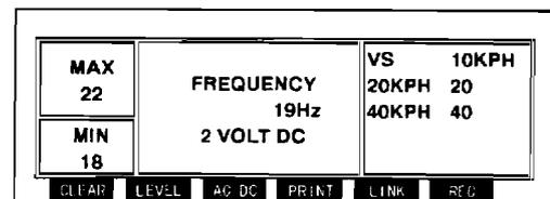
11. Press LEVEL key to change the threshold voltage to 6 VOLTS.
