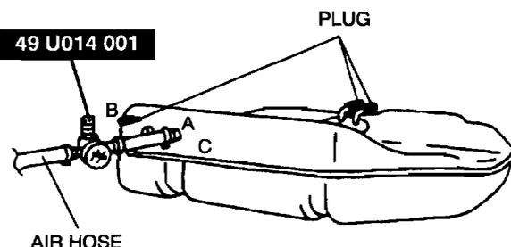
11. Apply pressure of **+0.98 kPa {+7.4 mmHg, +0.29 inHg}** to Port C and inspect if there is airflow from Port A.
