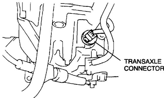
4. Measure the resistance between the terminals E and H.
