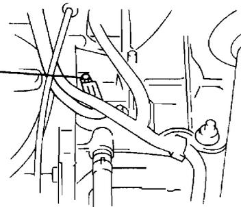
4. Measure the resistance between the terminals of the input/turbine speed sensor.
