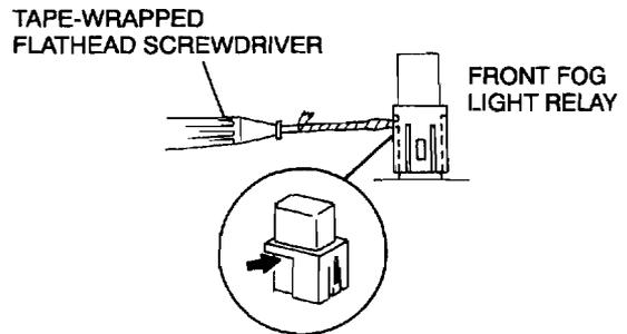
2. Pull out the front fog light relay while pressing the flathead screwdriver downward.
