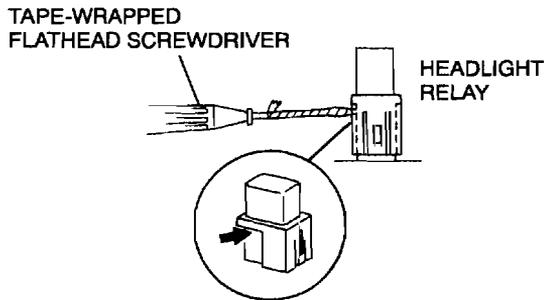
2. Pull out the headlight relay while pressing the flathead screwdriver downward.
