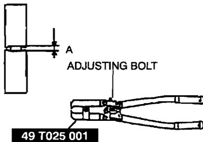
2. Crimp the wheel side small boot band using the SST. Verify that clearance B is within the specification.
