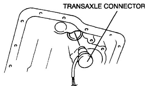
3. Remove the TFT sensor from the strainer, and connect it to the transaxle connector.
