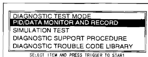
6. Access **RPM PID**. Press the trigger key to enter this selection. (See F1-33 PID/DATA monitor and record procedure.)
