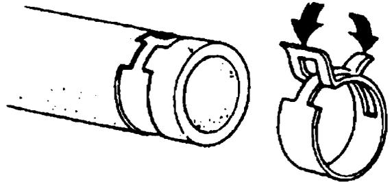
4. Verify that the hose clamp does not interfere with any other components.
