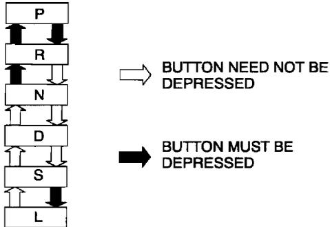
5. Verify that the positions of the selector lever and the indicator are aligned.
