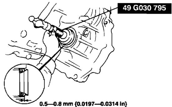
5. Coat the lip of the oil seal with transaxle oil.
