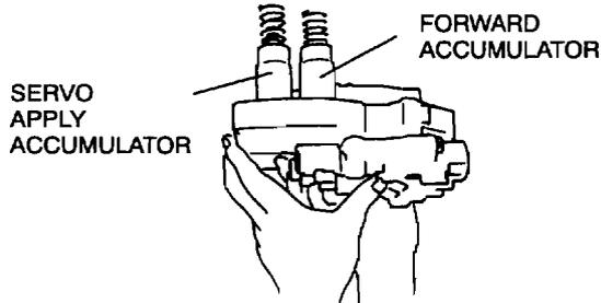
2. Install the control valve body component.
