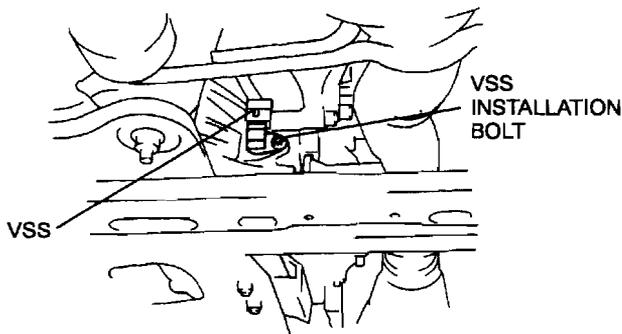
4. Apply ATF to a new O-ring and install it on a new VSS.
