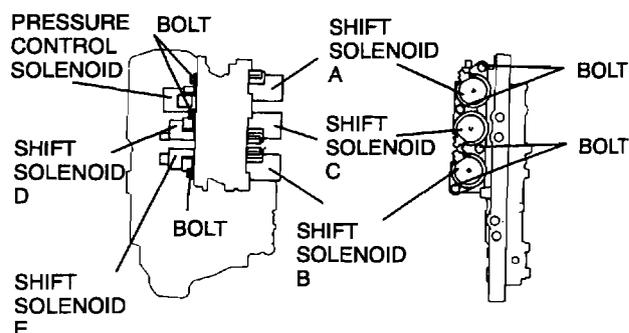
6. Install the control valve body. (See K2-46 CONTROL VALVE BODY INSTALLATION, On-Vehicle Installation.)
