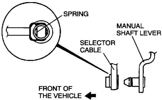
3. Install the selector lever to the manual shaft lever in such a way that the selector cable does not bear a load.
