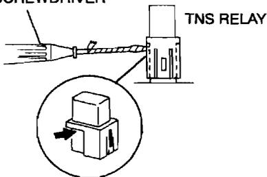
2. Pull out the TNS relay while pressing the flathead screwdriver downward.
