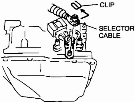
5. Rotate the manual shaft to the converter housing side fully, then return 2 notches to set the N position.
