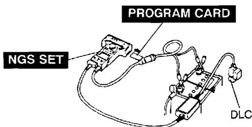
2. Select "VEHICLE & ENGINE SELECTION" and press TRIGGER. (Select the model and specifications of the vehicle you are testing.)
