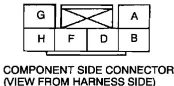
3. Apply 5 V to the power window motor terminal B and connect terminal F to ground.
