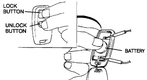
4. Measure the minimum voltage for a period of **10 seconds** from the time the transmitter buttons are pressed.
