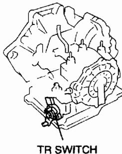
7. Loosen the TR switch mounting bolts.
