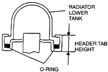
2. Insert the end of a medium tip screwdriver between the end of the header tab and the outer tank.
