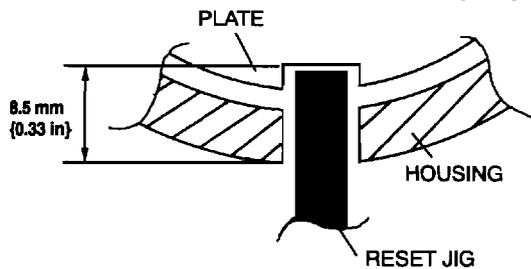
8. While inserting the reset jig to the end point, operate the power window switch to the open position so that the carrier plate moves to the lower end (below the motor).
