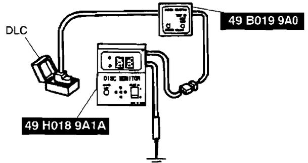
2. Set the select switch on the **SST** (self-diagnosis checker) to **A**.
