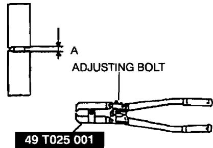
2. Crimp the band using the SST. Verify that clearance B is within the specification.
