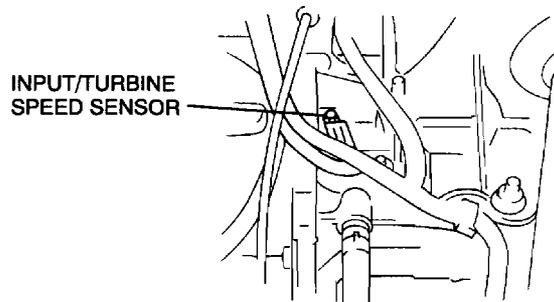
4. Remove the input/turbine speed sensor.
