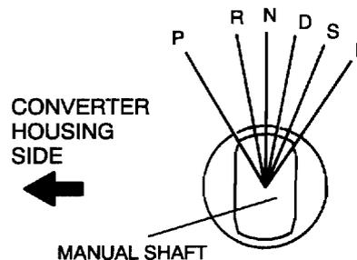
9. Align the protrusion and mark as shown.
