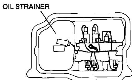
7. Remove the control valve body installation bolts A as shown, then remove the control valve body component as shown.
