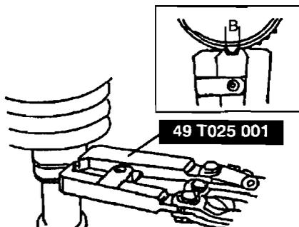
3. If clearance B is more than the specification, reduce clearance A of the SST and crimp the boot again.
