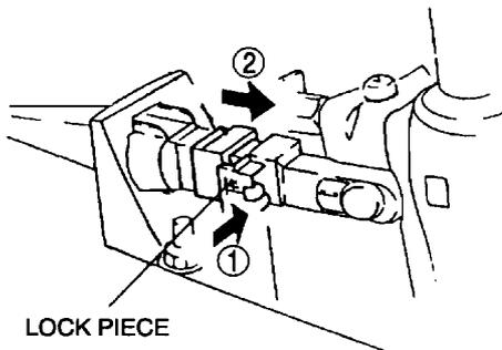
8. Shift the selector lever from P position to L range, and make sure that other components in that area do not interfere with the lever.
