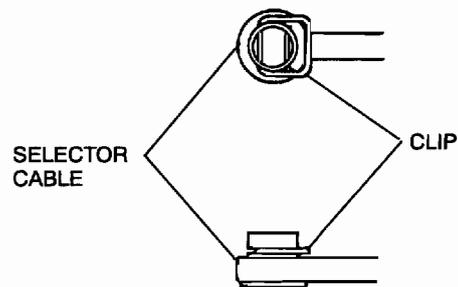
14. Connect the selector cable to the manual shaft lever as shown in the figure.
