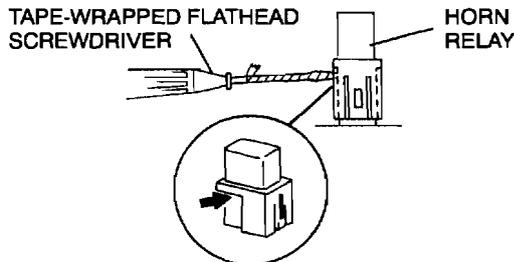
2. Pull out the horn relay while pressing the flathead screwdriver downward.
