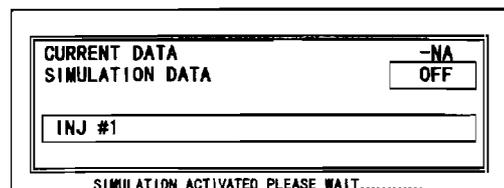
12. To perform the simulation again, press the **TRIGGER** key. To exit the idling test, press the cancel key.
