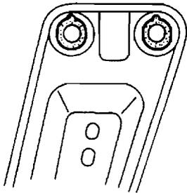
2. Install the No.2 engine mount to the transaxle.
